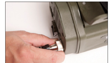
Hand-tighten connector collar.
